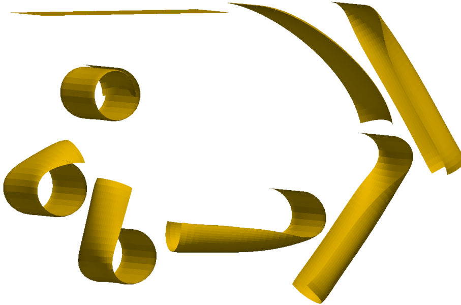
FIGURE 3. Pseudo-evolution (clockwise) towards the equilibrium of a clamped rectangular plate with spontaneous curvature Z = -I_2 . The bilayer plate is depicted (clockwise) for 0.0, 0.1, 2.4, 60.0, 100.0, 130.0, 135.0, 207.3 times 10^3 iterations of Algorithm 2. The bilayer plate reaches a cylindrical shape asymptotically (limit of discrete gradient flow). This is an absolute minimizer.
