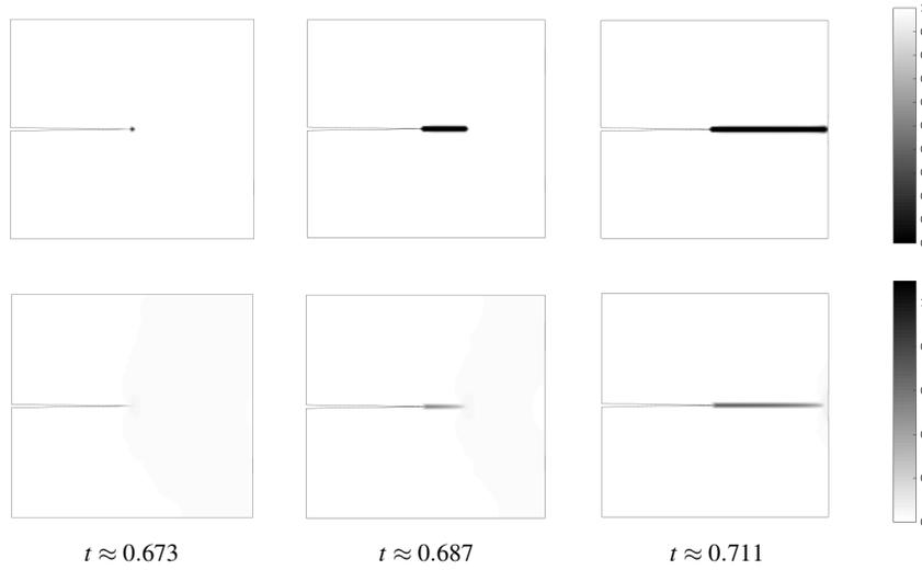
Fig. 7:  $H^1$ -regularized evolution for notched square with mesh size  $h_{\min} \approx 0.0078$  and time step size  $\Delta t = 1/1638$ . Top: Evolution of damage variable  $z$ . Bottom: Stress  $\sqrt{f(z)}e(u+g(t)) : \mathbb{C}e(u+g(t))$ .
