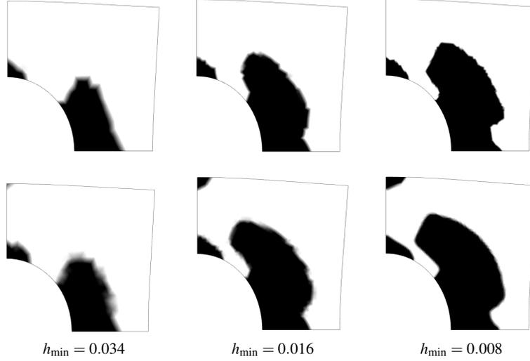
Fig. 3: Damage at  $t = 1$  for different mesh sizes and time step sizes. Top:  $BV$ -regularization. Bottom: Weighted  $H^1$ -regularization with  $\kappa h_{\min} \|\nabla z\|^2$ . Displacements are magnified by factor 40.
