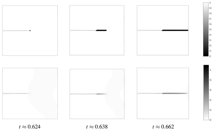
Fig. 6: *BV*-regularized evolution for notched square with mesh size  $h_{\min} \approx 0.0078$  and time step size  $\Delta t = 1/1638$ . Top: Evolution of damage variable  $z$ . Bottom: Stress  $\sqrt{f(z)e(u+g(t))} : \mathbb{C}e(u+g(t))$ .
