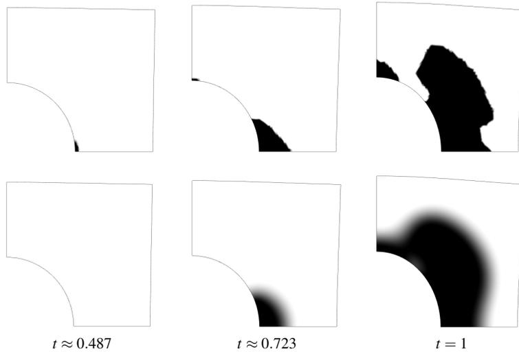
Fig. 2: Damage evolution with mesh size  $h_{\min} \approx 0.008$  and time step size  $\Delta t = 1/1492$ . Top:  $BV$ -regularization. Bottom: Unweighted  $H^1$ -regularization. Displacements are magnified by factor 40.
