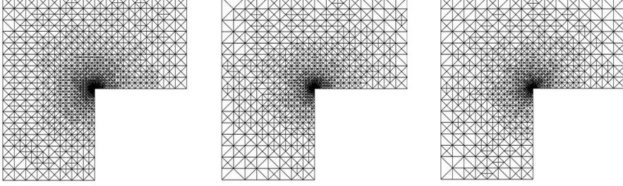
FIGURE 2. Snapshots of refined meshes for nonlinear Laplace problem with  $\sigma = 1.6$  (left),  $\sigma = 1.2$  (middle) and  $\sigma = 1.05$  (right). The mesh is locally refined in a neighborhood of the reentrant corner. The resolution at the reentrant corner increases as  $\sigma \rightarrow 1$ .
