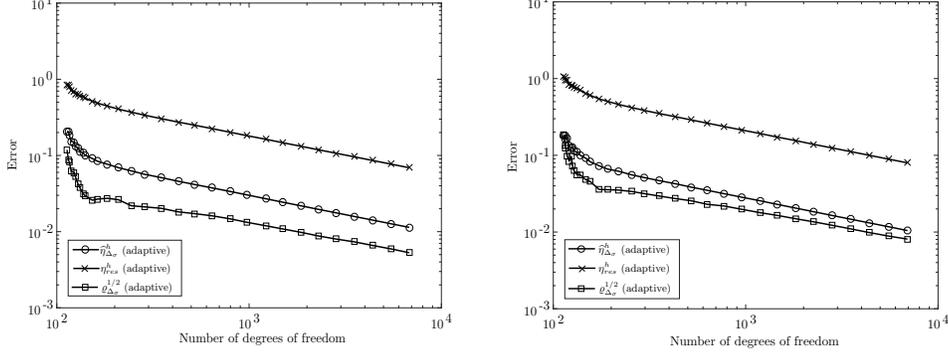
FIGURE 4. Primal-dual gap estimator  $\hat{\eta}_{\Delta\sigma}^h$ , residual-based estimator  $\eta_{res}^h$  and error  $\varrho_{\Delta\sigma}^{1/2} = \|V(\nabla u) - V(\nabla u_h)\|$  for a sequence of adaptively refined meshes driven by  $\hat{\eta}_{\Delta\sigma}^h$ . Left: Nonlinear Laplace problem with  $\sigma = 1.6$ . Right: Nonlinear Laplace problem with  $\sigma = 1.2$ .
