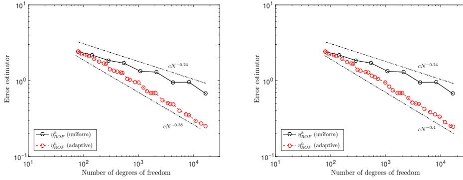
FIGURE 5. Error estimator  $\eta_{\text{rof}}^h$  for Example 6.1 with discretization of the dual problem with continuous finite element space  $Y_h^C$  (left) and  $H(\text{div}; \Omega)$ -conforming finite element space  $Y_h^{dC}$  (right) for uniform and adaptive mesh refinement.
