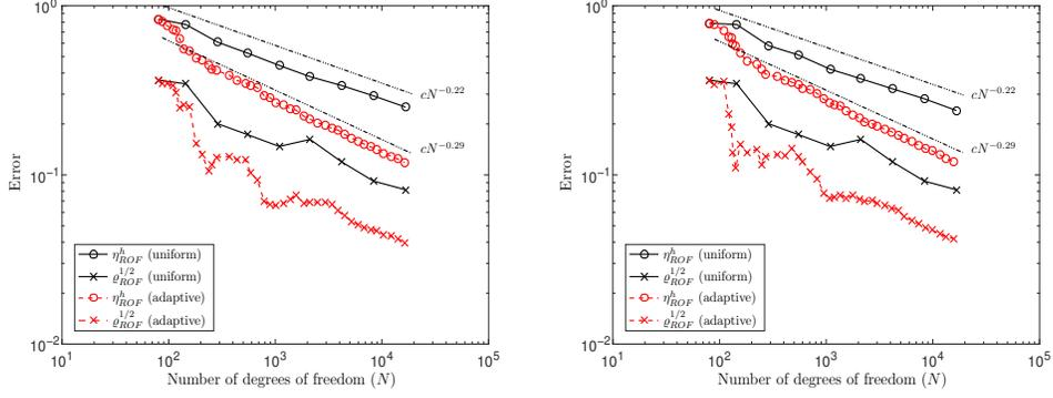
FIGURE 6. Primal-dual gap error estimator  $\eta_{\text{rof}}^h$  and  $L^2$ -error  $\varrho_{\text{rof}}^{1/2} = (\alpha/2)^{1/2}\|u - u_h\|$  for Example 6.2 with discretization of the dual problem with continuous finite element space  $Y_h^C$  (left) and  $H(\text{div}; \Omega)$ -conforming finite element space  $Y_h^{dC}$  (right) for uniform and adaptive mesh refinement.
