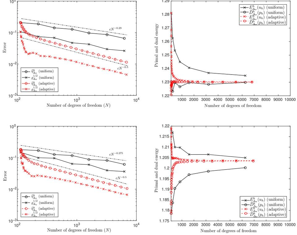
FIGURE 1. Primal-dual gap error estimators  $\hat{\eta}_{\Delta_\sigma}^h$  and error  $\varrho_{\Delta_\sigma}^{1/2} = \|V(\nabla u) - V(\nabla u_h)\|$  (left) and primal and dual energy  $E_{\Delta_\sigma}^h(u_h)$  and  $\hat{D}_{\Delta_\sigma}^h(p_h)$  (right) for uniform and adaptive mesh refinement. Top: Nonlinear Laplace problem with  $\sigma = 1.6$ . Bottom: Nonlinear Laplace problem with  $\sigma = 1.2$ .
