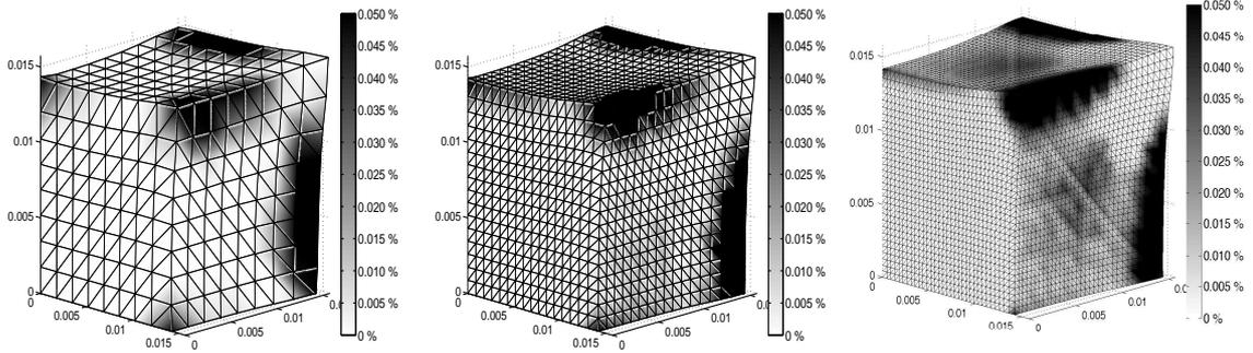
Figure 2: Postprocessed modulus of plastic strain  $|\pi_{\tau h}(t, \cdot)|$  for  $t = t_* = 0.075\text{s}$  and the mesh sizes  $h = 2^{-\ell}\sqrt{3}10^{-2}\text{m}$ ,  $\ell = 3, 4, 5$  (from left to right). The finest mesh has 163 840 tetrahedral elements.
