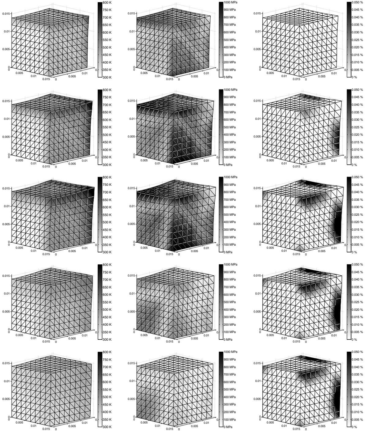
Figure 1: Displacement (magnified by factor 60) together with temperature  $\theta_{\tau h}(t, \cdot)$ , postprocessed modulus of stresses  $|\sigma_{\tau h}(t, \cdot)|$ , and postprocessed modulus of plastic strain  $|\pi_{\tau h}(t, \cdot)|$  (from left to right) for  $t = 0.025, 0.05, 0.075, 0.15, 0.3$ s (from top to bottom) with  $f$  defined through (5.6) with  $t_* = 0.075$ s.
