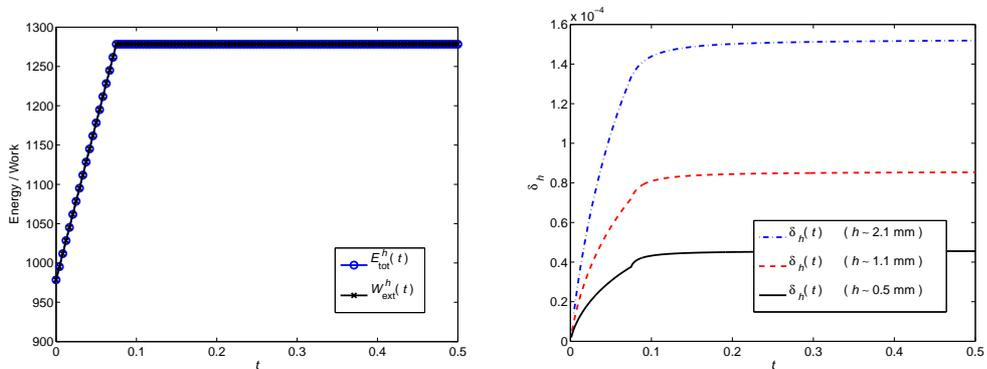
Figure 3: Total discrete energy and work of external heat (left). The relative difference between the total discrete energy and the external forces is small and converges linearly to zero as  $h \rightarrow 0$  (right).
