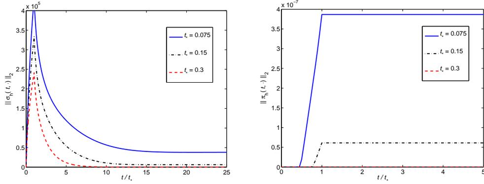
Figure 4:  $L^2$  norms of discrete stresses (left) and plastic strains (right) as functions of the relative time  $t/t_*$  for heating times  $t_* = 0.075, 0.15, 0.3$ s. The plastic material behaviour becomes less pronounced as the external heating happens slower.
