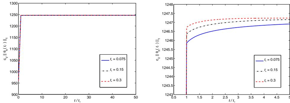
Figure 5: Thermal part of the energy for different speed of the heating regimes given by (5.6) for  $t_* = 0.075, 0.15, 0.3$ s. The detailed picture (right) shows that final temperature is slightly lower if the material was more plasticized during the heating.
