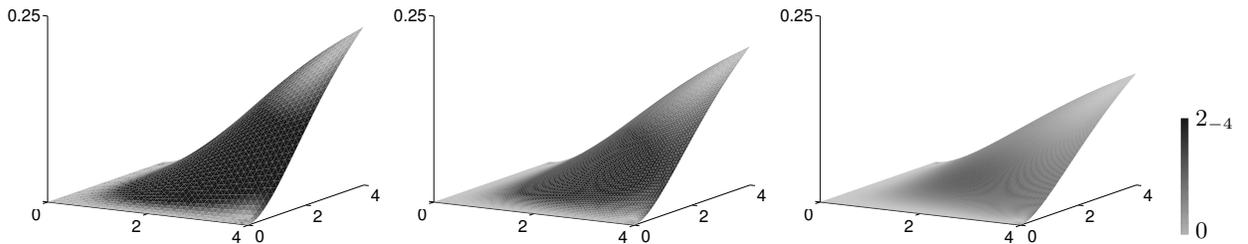
FIGURE 2. Discrete deformations of a clamped  $4 \times 4$  plate subject to a uniform vertical load and modulus of corresponding discrete Gaussian curvature on the triangulations  $\mathcal{T}_3$ ,  $\mathcal{T}_4$ , and  $\mathcal{T}_5$  in Example 4.1.
