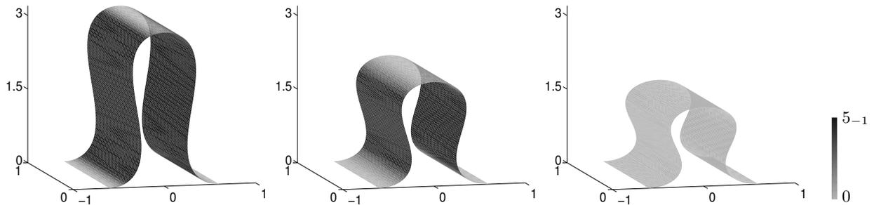
FIGURE 4. Discrete deformations for the compression of a  $4 \times 1$  plate with a small uniform vertical load on the triangulation  $\mathcal{T}_5$  obtained with the time-step size  $\tau = \widehat{h}^\beta$  for  $\beta = 0.5, 1.0, 1.5$ . The deformations are colored by the error  $\delta I_h$ .
