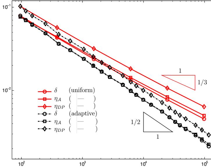
FIGURE 1. Error  $\delta = \|\nabla(u - u_h)\|$  and error estimators  $\eta_A$  and  $\eta_{DP}$  versus degrees of freedom  $N$  for a Poisson problem on an  $L$ -shaped domain defined in Example 5.1 for uniformly and adaptively refined triangulations. All quantities decay with the same rates  $N^{-1/3}$  and  $N^{-1/2}$  for uniform and adaptive mesh-refinement, respectively.
