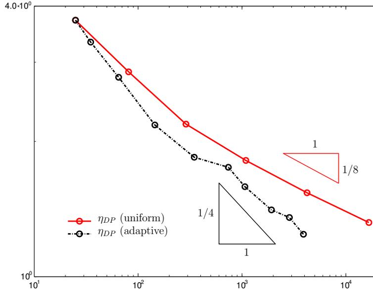
FIGURE 3. Error estimator  $\eta_{DP}$  versus degrees of freedom  $N$  for the total variation minimization problem defined in Example 5.3. The estimator decays at a rate  $N^{-1/8}$  for uniform refinement. The numbers are reduced on adaptively refined meshes with comparable numbers of degrees of freedom and the rate is improved to  $\eta_{DP} \sim N^{-1/4}$ .
