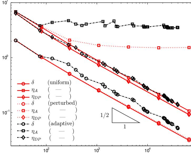
FIGURE 2. Error  $\delta$  and error estimators  $\eta_A$  and  $\eta_{DP}$  versus degrees of freedom  $N$  for a Helmholtz type problem on a square defined in Example 5.2 for uniformly, perturbed uniformly, and adaptively refined triangulations. The reliable estimator  $\eta_{DP}$  decays at the same optimal rate as the error on all sequences of triangulations while the reliable estimator  $\eta_A$  is efficient only on uniformly refined, highly symmetric triangulations.
