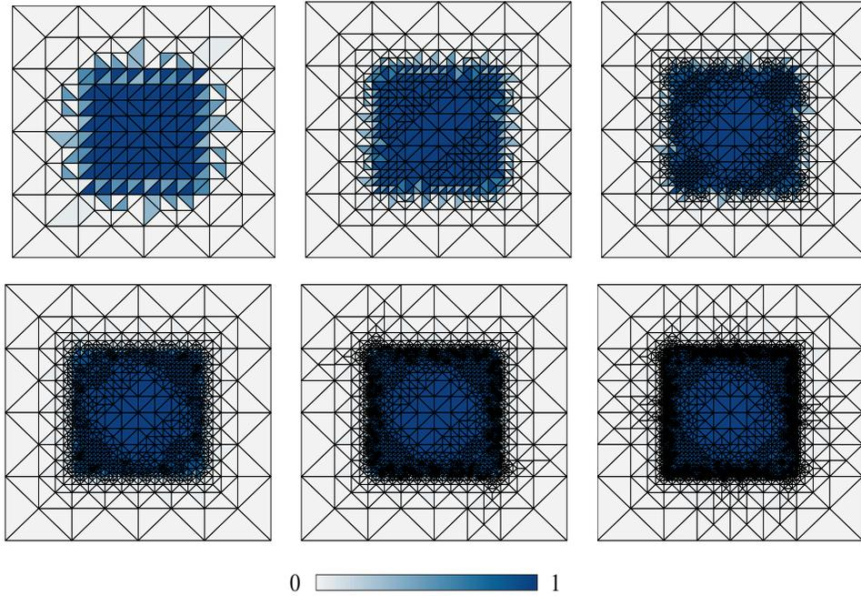
FIGURE 4. Adaptively generated grids and numerical solutions  $u_h$  in Example 5.3. The adaptive strategy steered by the refinement indicators  $\eta_{DP}(T)$  automatically refines a neighbourhood of the discontinuity set of the data function  $g$  which is expected to coincide with the singularity set of the exact solution  $u$ .
