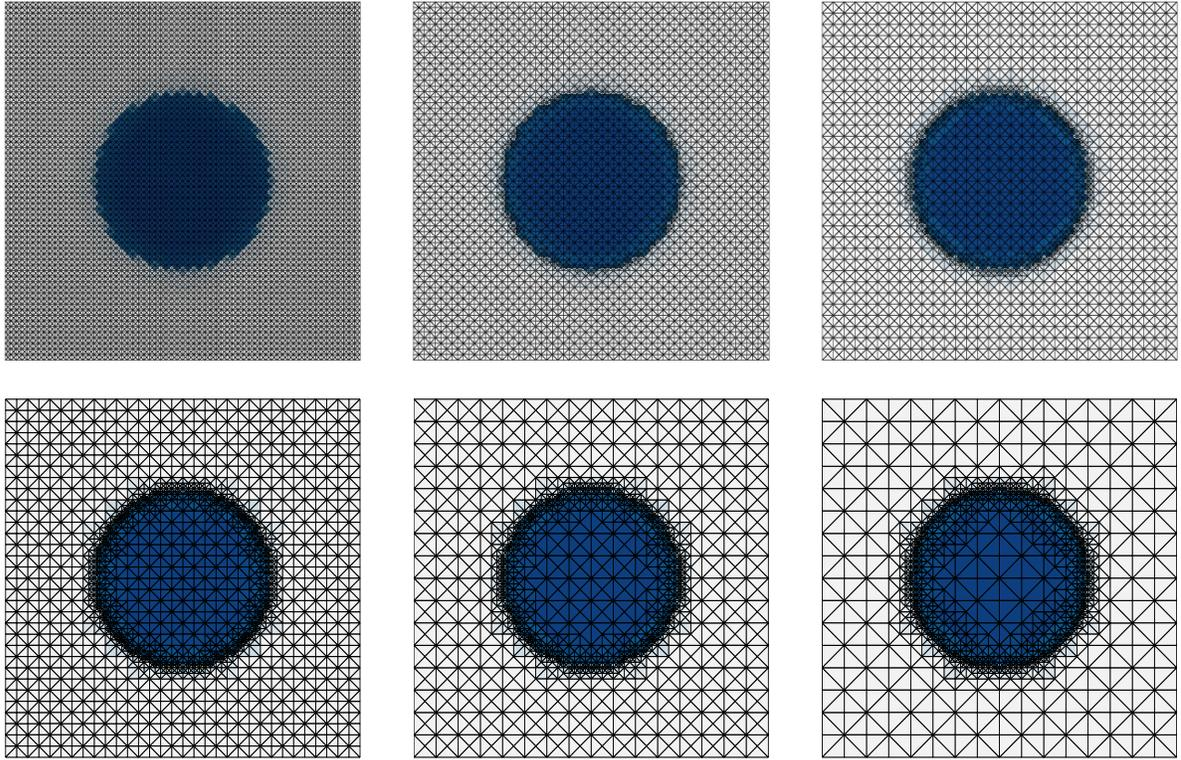
FIGURE 5. Adaptively refined and coarsened grids and numerical solutions  $u_h$  in Example 5.4. The mesh is significantly coarsened away from the circular discontinuity set and refined therein.
