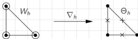
**Discrete gradient:**  $\nabla_h$  for  $w_h \in W_h$  defined as  $\theta_h = \nabla_h w_h \in \Theta_h$  via
